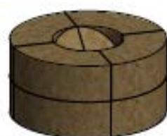
... then the second layer is completed with two segment heat-storing bricks.
