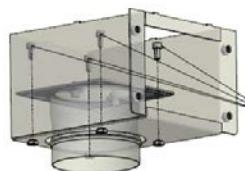
The feed air box panel, together with the feed air connection which has now been screwed to it, is now refitted to the feed air box floor with 4 screws.
