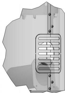
These webs have to be cut through and the panel has to be removed so that a feed air duct can be fitted to the feed air connection from the rear.
